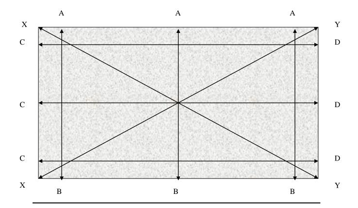
TOLERANCE MEASURED ACROSS 1400MM WIDTH (A-B) ≤ 1.5MM
